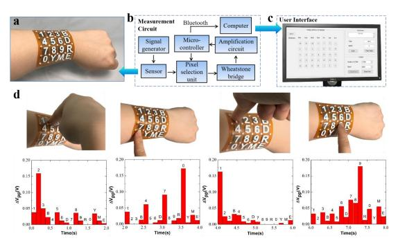
**Figure 6.** Demonstration of the utility of the flexible inductive pressure sensor array. (**a**) A wearable sensor prototype is attached on the forearm, in which each unit corresponds to a unique character. (**b**) The schematic illustration of the measurement circuit system. (**c**) A programmable user-interface display in a PC. (**d**) The voltage changes when four units of '2', '0', '1' and '9' are pressed by the fingertip.
