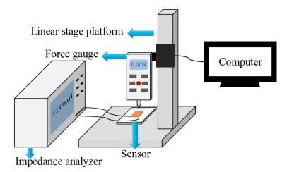
Figure 2. The measurement setup for the device calibrations.
